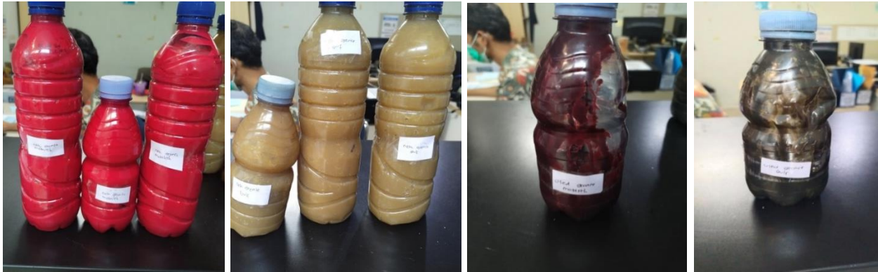
Figure 2. (a) Sample of New Mobilith SHC 100 (b) Grease Sample of New Gulf Crown EP 2 Grease (c) Sample of Used Mobilith SHC 100 Grease (d) Sample of Used Gulf Crown EP 2 Grease
