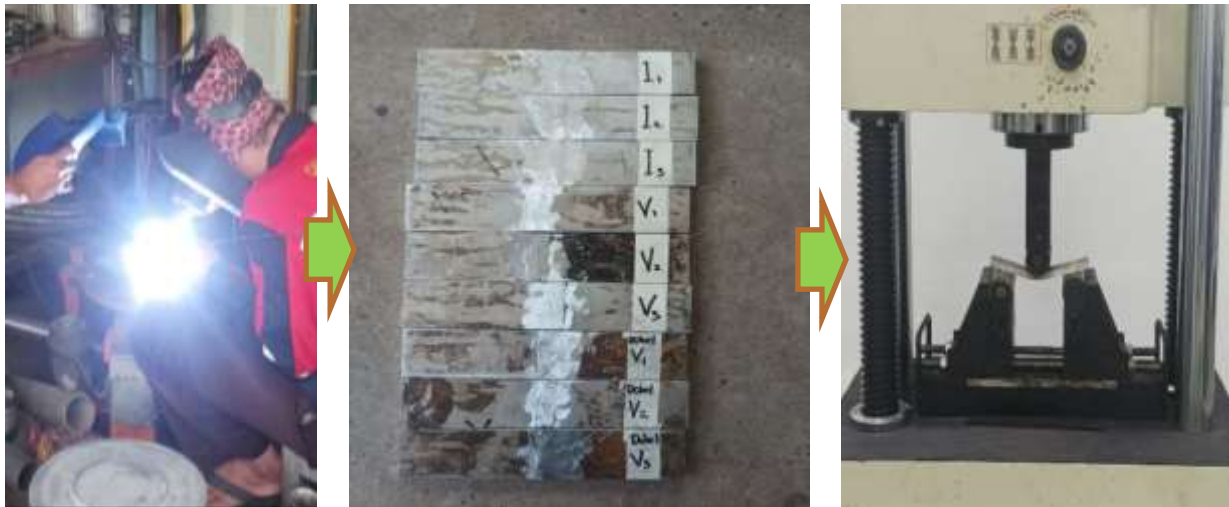
Figure 2. Welding and Speciment Testing
