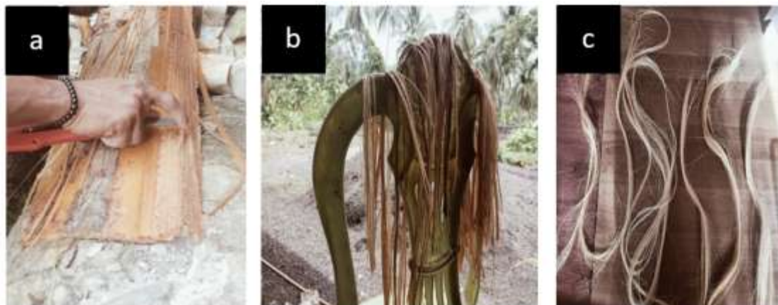
Figure 1. Banana stem fibers: (a) BSF shredding process, (b) BSF drying and (c) purified BSF
